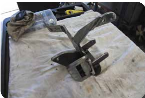
Montagesteun tbv aircopomp.
