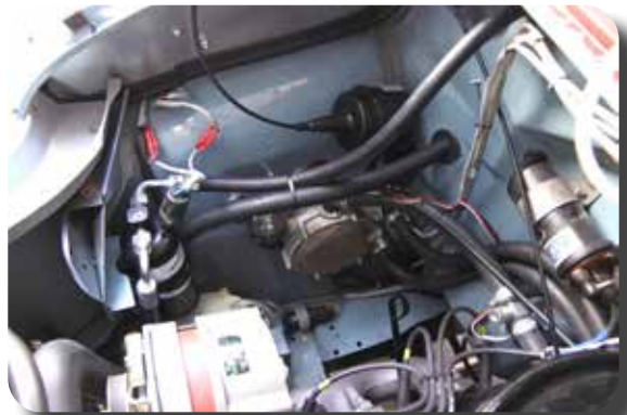
Airco droger, cruise-control, LPG instalatie.
